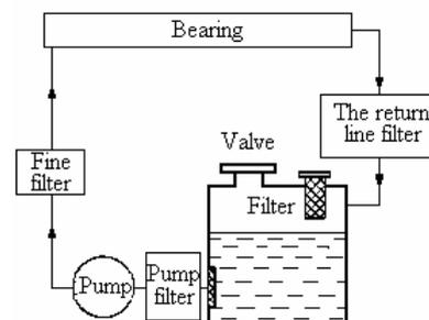
**Fig. 3.** The principle scheme a filtration system [2]
