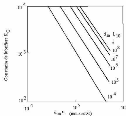
Fig. 1. Constant value when using grease lubrication [1]
